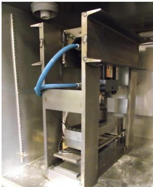
**Test Setup for Calibration Derivation in Oven**
