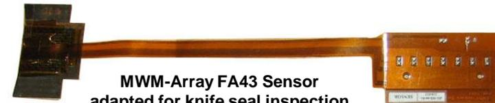
MWM-Array FA43 Sensor adapted for knife seal inspection
