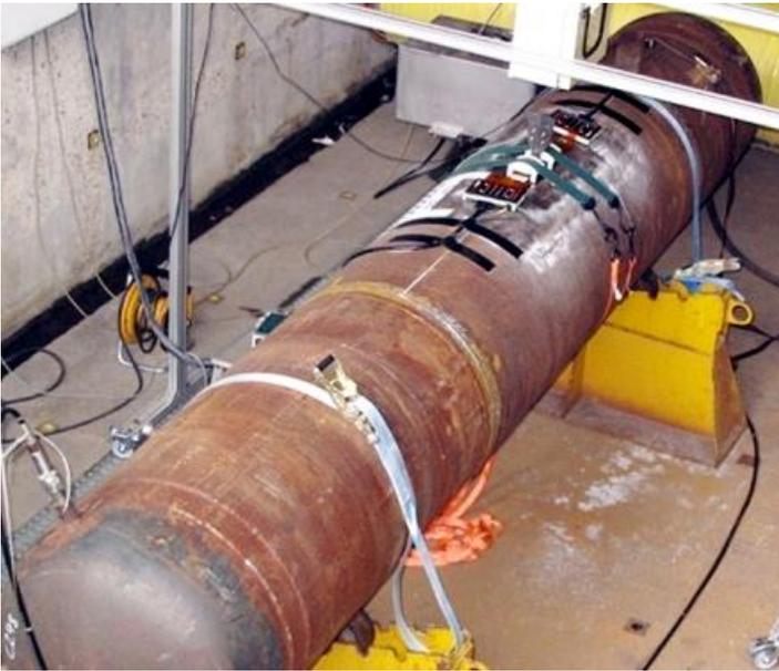
**PHOTOGRAPH GDF TEST SETUP FOR CRACK GROWTH AND STRESS MONITORING USING AN INSTALLED MWM-ARRAY AT A MECHANICAL DAMAGE SITE**
