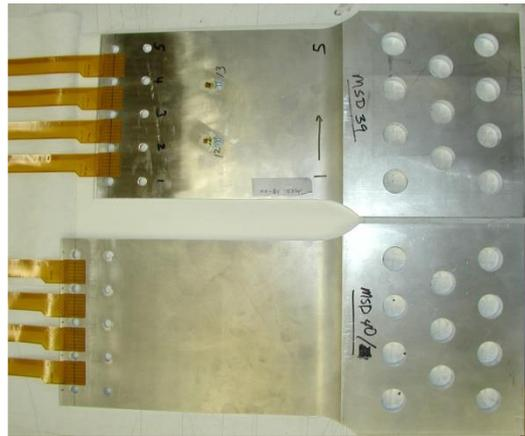
**10-Hole Specimen with MWM-Array Networks**
